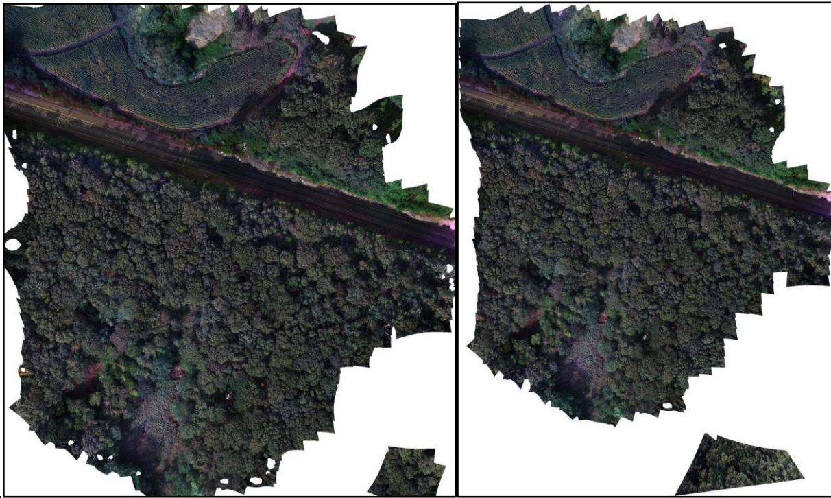
Orthomosaics for Flight 1 without (left) and with XMP data (right).
